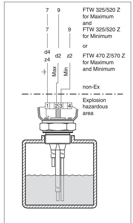
Independent two limit detection in a plastic vessel without cable monitoring and also for use in explosion hazardous areas
