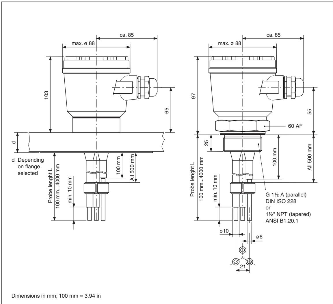
Dimensions of the three-rod probes 11363 and 11363 Z. Height and diameter are similar for all housings.
