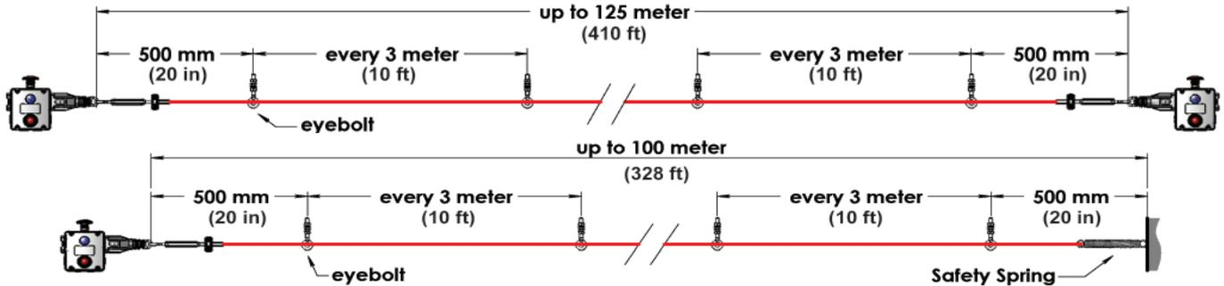
It is important that the first 500mm is not used as part of the active protection coverage. If protection is required in this first 500mm then it is recommended to use switches fitted with a mushroom type E-Stop button. IDEM also recommend when using a Safety Spring that a maximum of one corner pulley is used.
