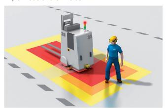
Two field set modes can be selected with S3000 Expert. With triple mode a second warning field is available. Thereby pedestrians passing by an automated guided vehicle could be warned with an acoustic sound and additionally by a visual signal when being further approached by the vehicle. The dual-field mode with only one warning field can be also selected.
