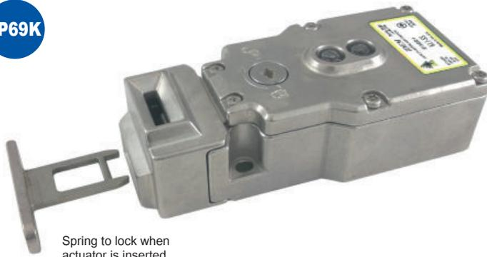
Spring to lock when actuator is inserted. Energise solenoid to unlock.
