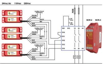
Three switches connected in series to an SCR-2 or SCR-3 to give Dual Channel guard monitoring with Automatic Start and Contactor Feedback check
