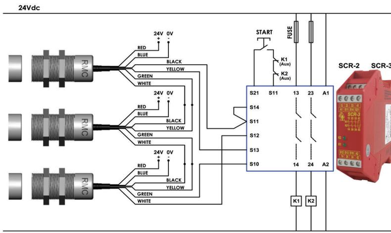
Three switches connected in series to an SCR-2 or SCR-3 to give Dual Channel guard monitoring with Manual Start and Contactor Feedback Check.
