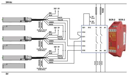
Three switches connected in series to an SCR-2 or SCR-3 to give Dual Channel monitoring with Automatic Start and Contactor Feedback Check. Optional auxiliary circuits provide for remove signalling from each switch.
